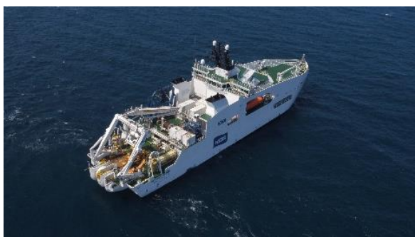
Submarine cable laying ship (Courtesy: Kokusai Cable Ship Co., Ltd.)
