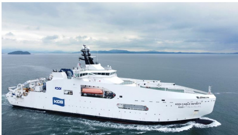
Subsea cable-laying ship KDDI Cable Infinity
