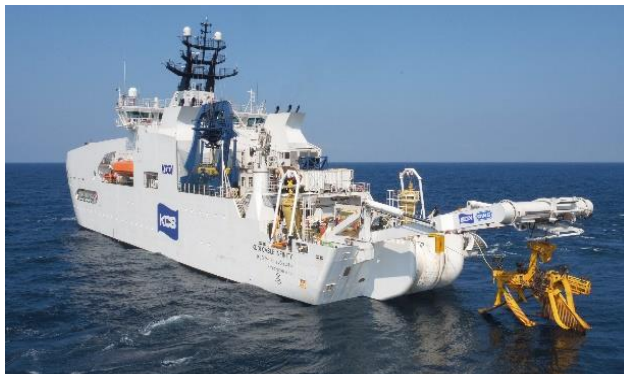
Cable Laying Vessel (Photo courtesy: KDDI Cablesheets & Subsea Engineering Inc.)
