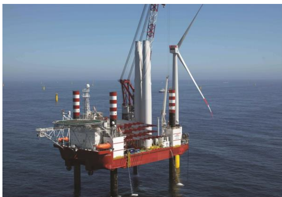
洋上風力発電設備設置船 Self-Elevating Platform (写真提供：Seajacks Japan Ltd)
