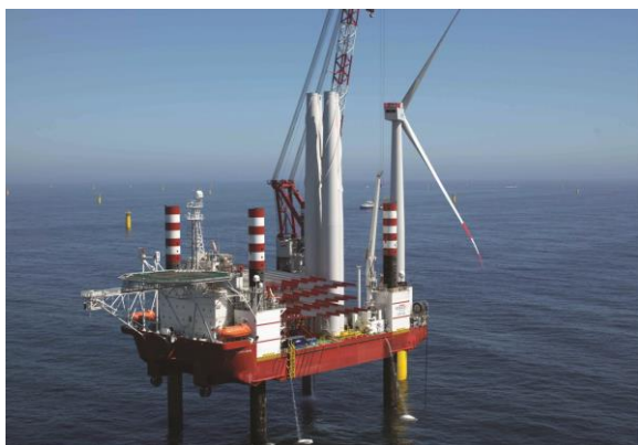
洋上風力発電設備設置船 Self-Elevating Platform (船名:Wind Zaratan)
